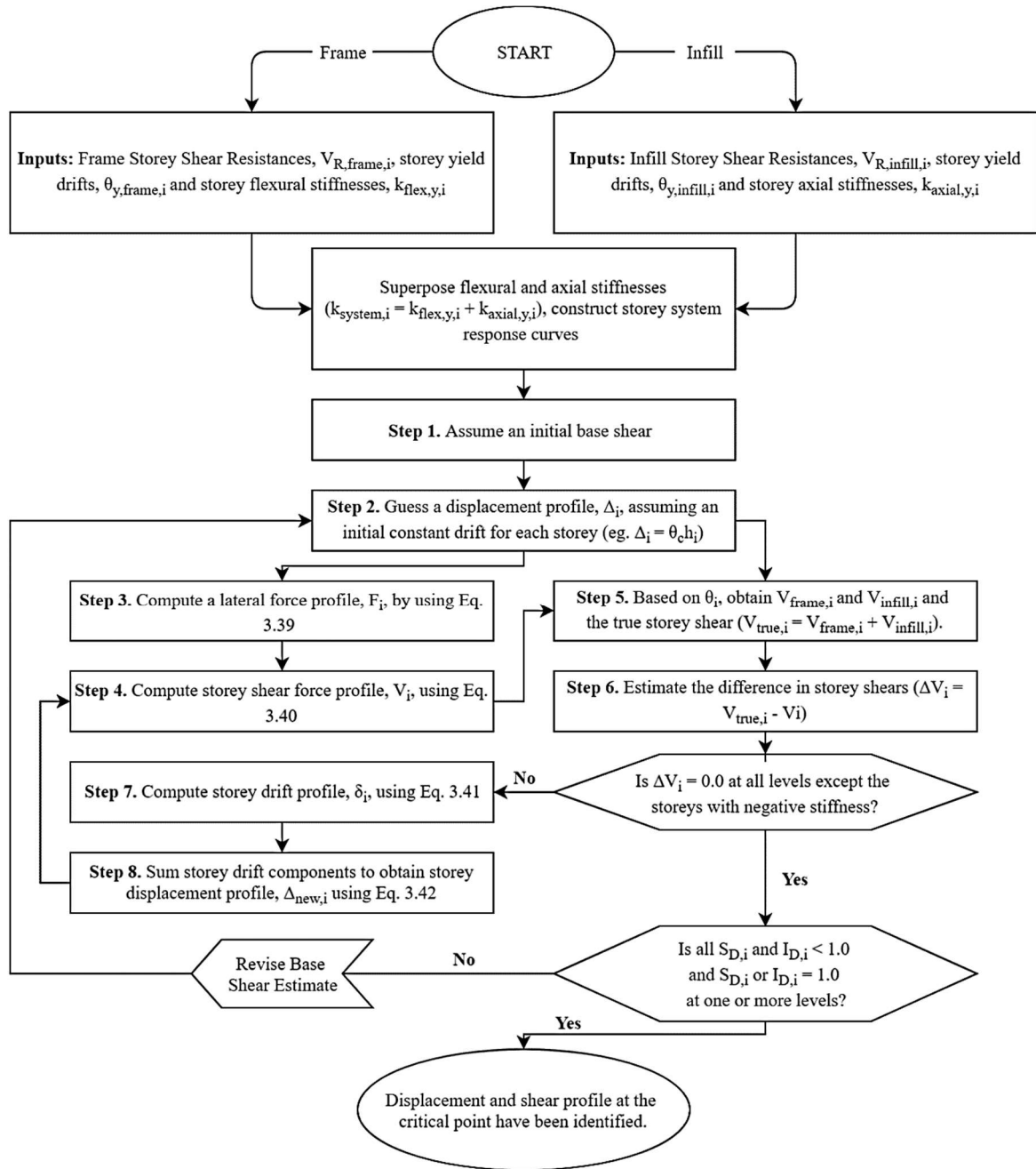
Figure 3.11. Flowchart of the proposed simplified analysis procedure.
